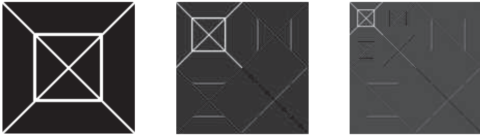
Figure 5.5: 2D discrete wavelet transform of a test image. On the left hand side the original image is shown, in the middle the first level decomposition and on the right the second level. The image is transformed with Daubechies D4 filter, see section 5.3.1.
