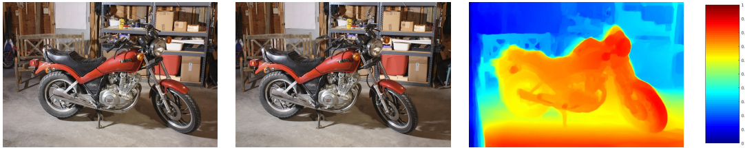
Figure 4: Stereo Matching. The two images on the left are the input images. They were taken from slightly different viewpoints and have already been rectified. Right image: Depth map as found by minimizing the stereo matching problem. Warm colors indicate regions that are close to the camera position, cold colors indicate regions that are further away. Source of input images: (SHK + 14). The picture on the right was calculated for this thesis using Matlab and the libraries prost and sublabel_relax (MLM + 15).
