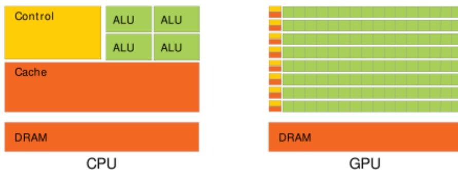
Figure 8: Schematic design of a CPU and GPU. Whereas the CPU devotes a large portion of transistors to flow control and data caching, the GPU provides more arithmetic logic units (ALUs) needed for data processing [43].
