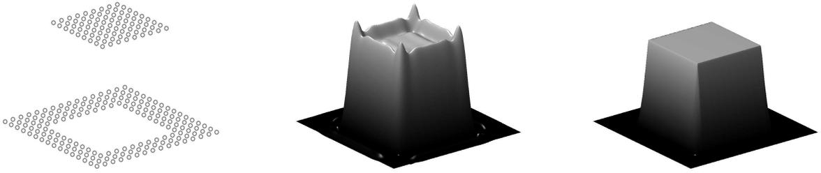
Figure 4. The interpolated data values (left) and the cubic B-Spline interpolant (middle) as well as the linear interpolant (right) is shown. Note the ringing in the B-Spline interpolant.
