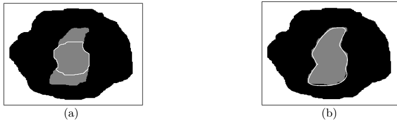
Figure 4. (a) start contour, (b) contour obtained by the GVF approach.
